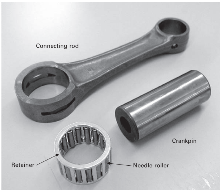
9.1 Monolithic con-rod. The lower left shows a needle roller bearing held in the retainer.
