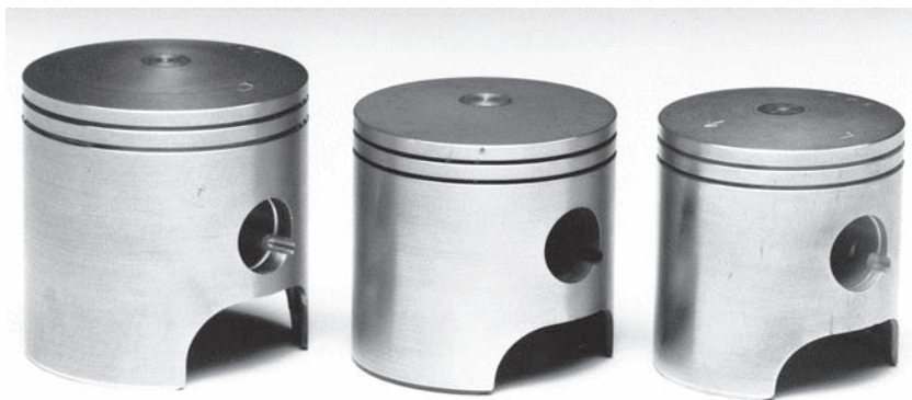
3.2 Two-stroke engine pistons made of a powder metallurgical aluminum alloy. Two-stroke engines normally install two piston rings (Chapter 4). The long skirt is necessary for exchanging gas.
