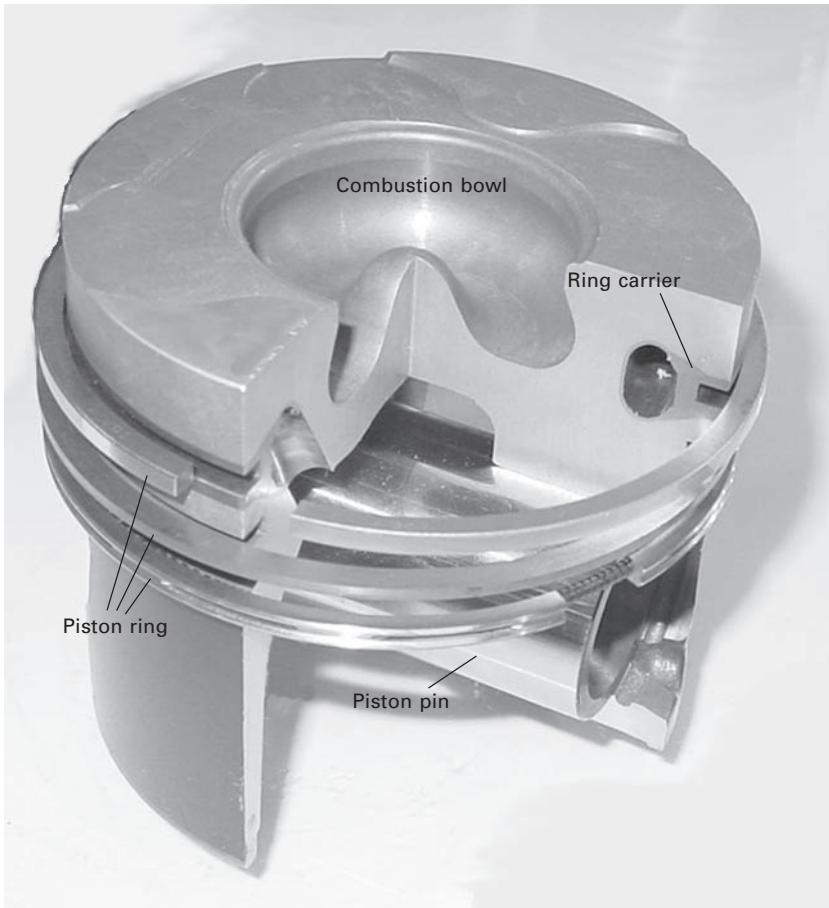
3.6 Aluminum piston for a direct injection diesel engine. The edge of the combustion bowl is fiber-reinforced. The top ring groove is reinforced with a Niresist ring carrier.
